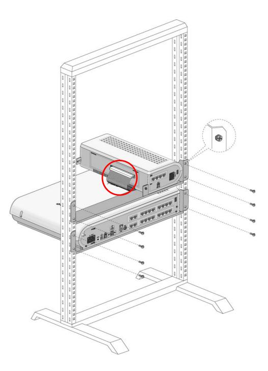
Figure 4.3.3.4 Module Rack Mounting
